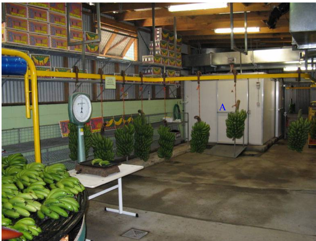
Figure 4. Packing shed in a small commercial facility showing cool room (A), harvested bunches hanging on a conveyor system, and turntable (left foreground) for washing individual hands removed from the bunches. [Photo credit: Janet Gorst, OGTR]
