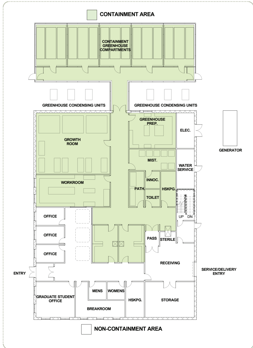
FIGURE 7. Typical Containment Facility Floor Plan*
